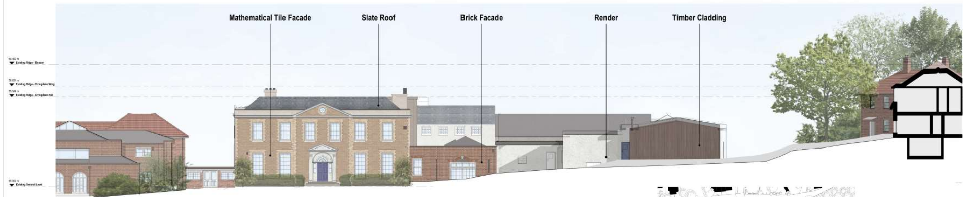
2 BB - Existing South Elevation 1:50
